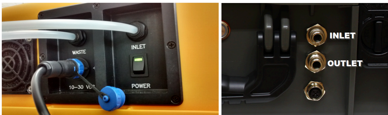
Figure 12. Left: Inlet and Waste push-connect ports on the U-GGA. Right: Inlet (top) and outlet (bottom) ports on the eosMX-16.
