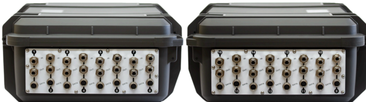
Figure 6. The eosMX-16 side panels, showing chamber tubing Inlet/Outlets and Data ports 1 through 8 (left) and 9 through 16 (right)
