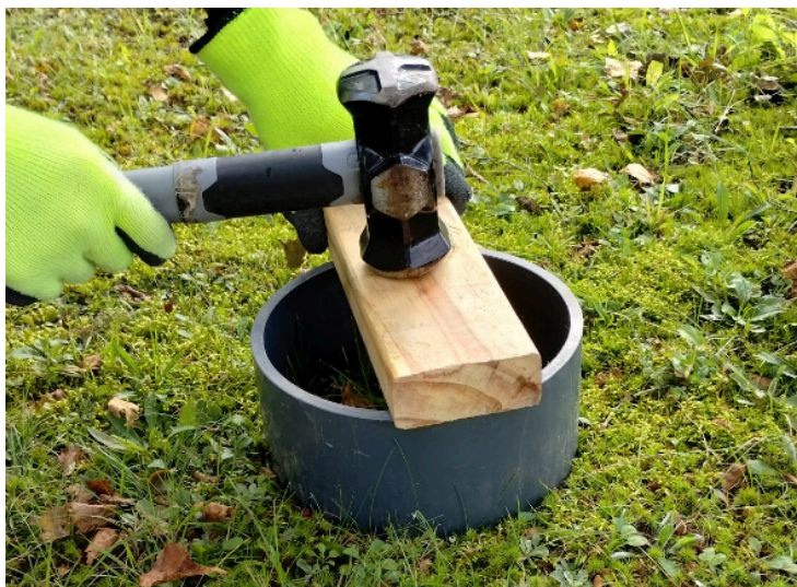
Figure 3. (left) Collar insertion into soil, applying force evenly using a hammer and wood, (right) chamber installation after collar insertion
