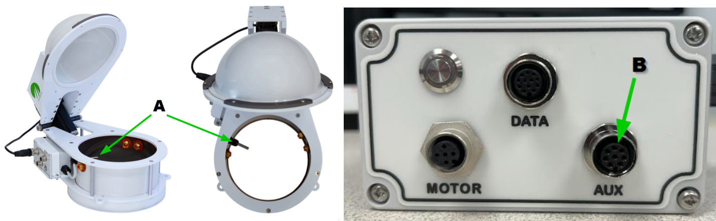
Figure 2. eosAC-T/O sensors: (A) temperature sensor, (B) exterior auxiliary port.
