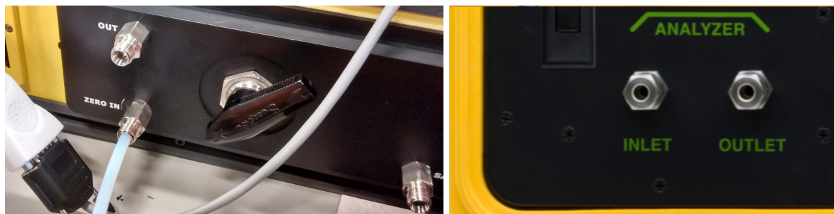
Figure 16. Left: Out, Zero In and Sample ports on the DX4015. Right: Inlet (left) and outlet (right) ports on the eosMX-P.
