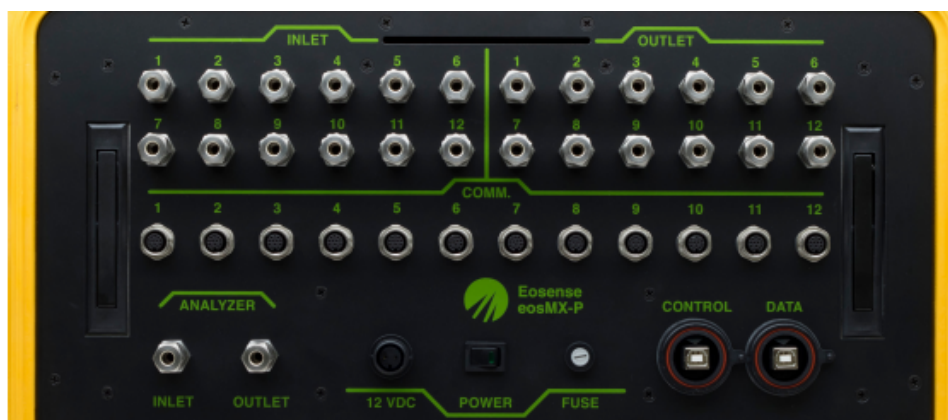
Figure 8. The eosMX-P face, showing chamber tubing inlet/outlets and COMM ports (top), the gas analyzer Inlet and Outlet ports (bottom-left), the power cable port and On/Off switch (middle), and the USB ports (bottom-right).
