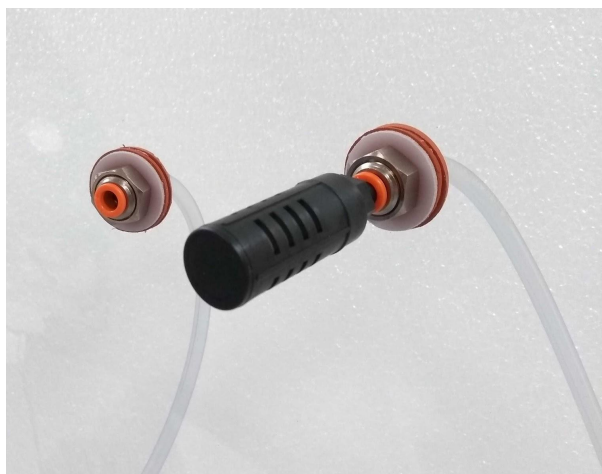
Figure 5. Gas muffler installed on Inlet.
