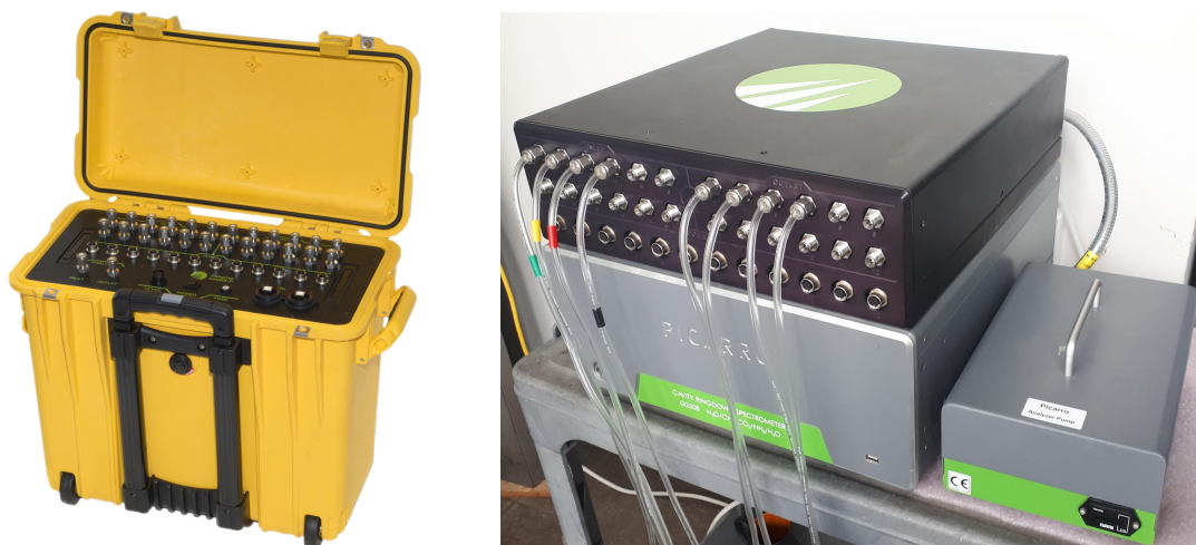
Figure 6. eosMX-P hard portable case (left) and an eosMX stacked on top of a Picarro analyzer (right).
