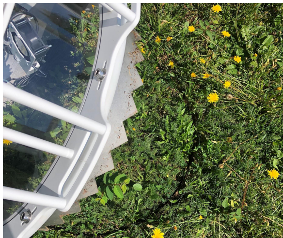
Figure 4. Circle pre-cut into soil for collar, which is installed securely on chamber in the field.
