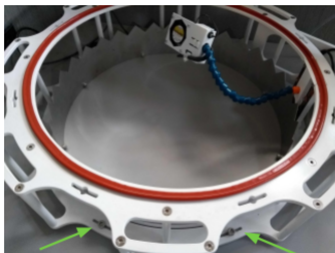
Figure 3. The collar (10 cm) comes installed inside the chamber. Green arrows point to 2 of 8 bolts that need to be removed upon receiving a new eosAC-LT/LO chamber (left). The provided collar seal should be installed by the user before deployment (right).
