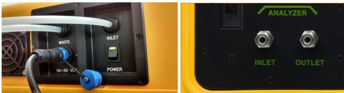
Figure 15. Left: Inlet and Waste push-connect ports on the U-GGA. Right: Inlet (left) and outlet (right) ports on the eosMX-P.
