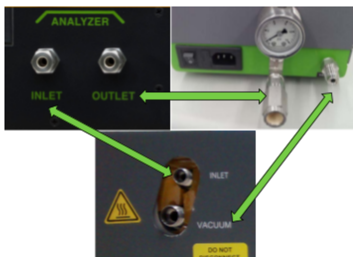
Figure 12. Gas tubing connections between the eosMX-P (top-left), external pump (top-right), and Picarro analyzer (bottom).
