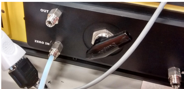
Figure 1. Out, Zero and Sample ports on the DX4015 gas analyzer.
