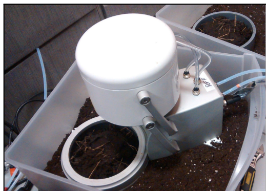
Figure 11. An eosAC sitting on the prepared soil plot, plumbed to the eosMX and Gasmeter DX4015 analyzer.
